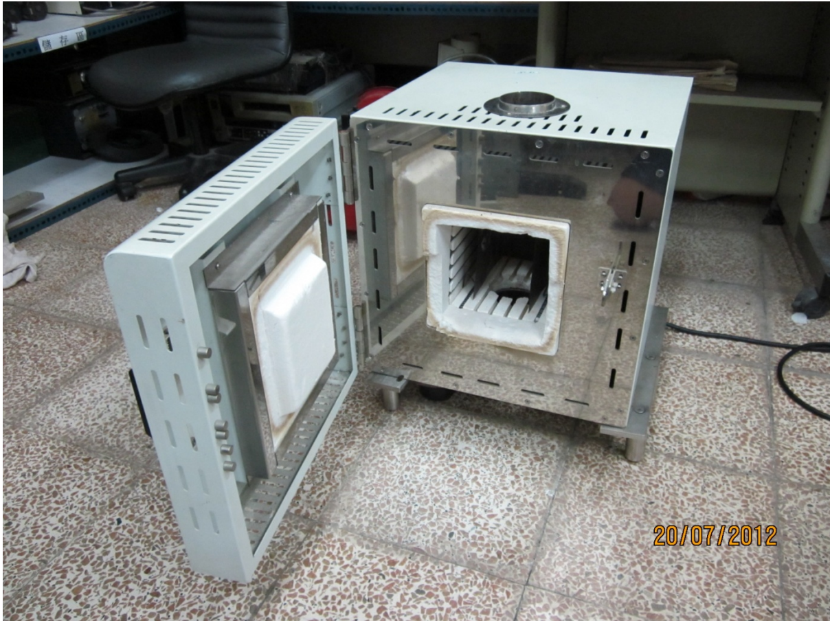
Figure 2-3 The picture of three-zone high temperature furnace attached to the Universal Testing Machine Instron 5582.
